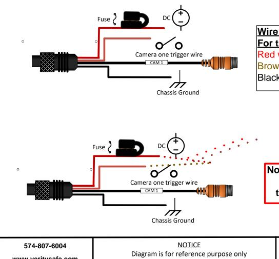
Wire Connection Key For trucks that cannot be shut off in reverse: Red wire to Ignition hot (+) 10-24v. DC Brown trigger wire for camera 1 Black wire to ground block or ground post GND (-)
